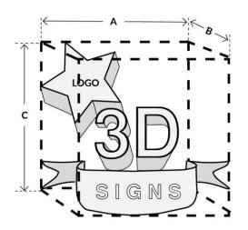
Sign area is computed using the smallest rectangular prism that will encompass the entire sign.
