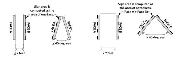
FIGURE 18.18.050.A.2: MEASURING SIGN AREA, DOUBLE-FACED SIGNS
