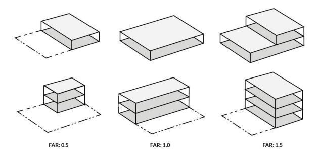
FIGURE 18.02.030.F: DETERMINING FLOOR AREA RATIO
