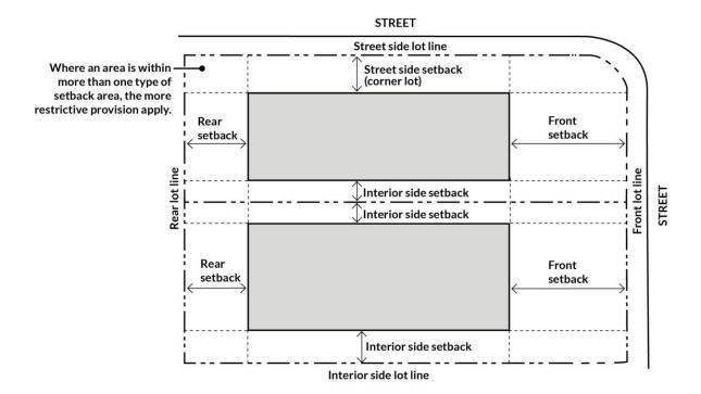
FIGURE 18.02.030.I: DETERMINING SETBACKS
