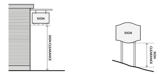
FIGURE 18.18.050.C: MEASURING SIGN CLEARANCE
