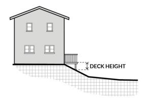
FIGURE 18.02.030.C.2: MEASURING HEIGHT OF DECKS
