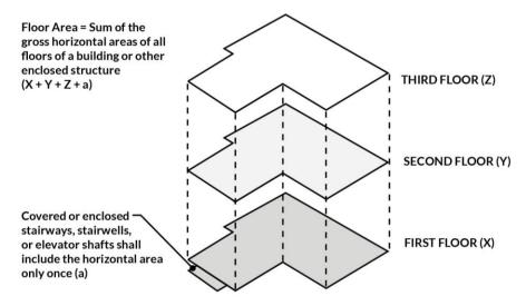
FIGURE 18.02.030.E: DETERMINING FLOOR AREA
