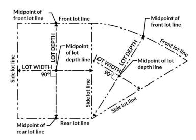
FIGURE 18.02.030.D: MEASURING LOT WIDTH AND DEPTH
